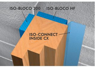
Installation example: ISO3-WINDOW SEALING SYSTEM
