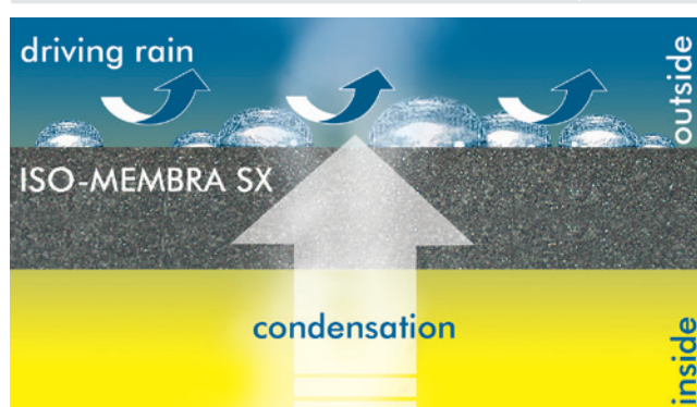
Performance principle of membrane seal
